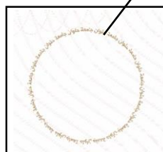
Fig 8: illustrates microprinting in The circle designed as guide to print the "Eagle Stamp"
