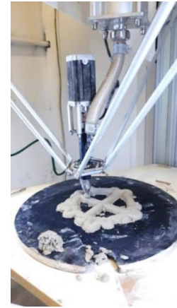
Fig. 12 Printing Process Courtesy of the Author
