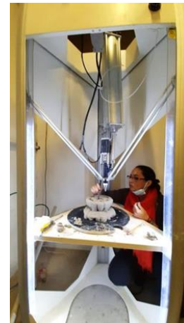
Fig. 13 Removing excess material Courtesy of the Author
